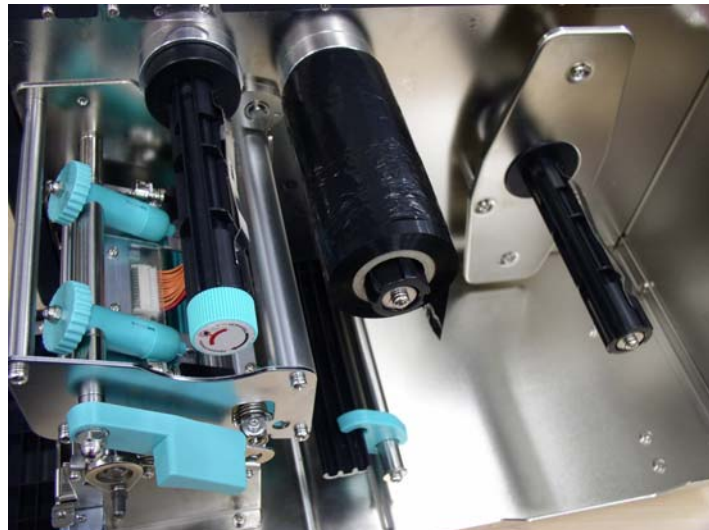
Figure 5. Ribbon supply spindle installation
